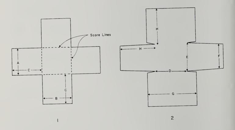
Fig. 1) Outline of chipboard box; 2) Outline of cover paper (dimensions given in table).
